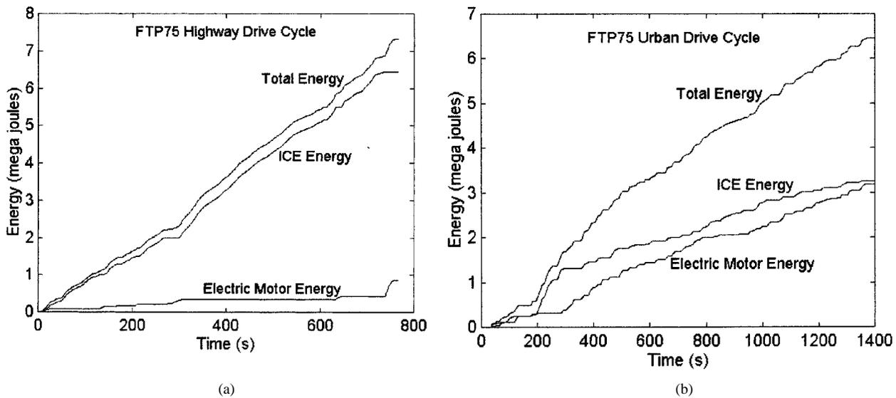
Fig. 6. Energy consumption in HEV for (a) highway and (b) urban drive cycles.
