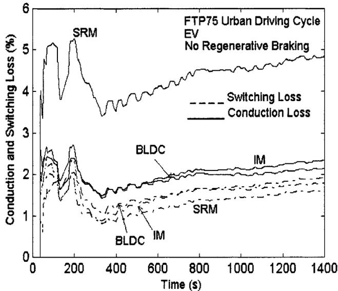
Fig. 9. Converter losses for EV in urban drive cycle.
