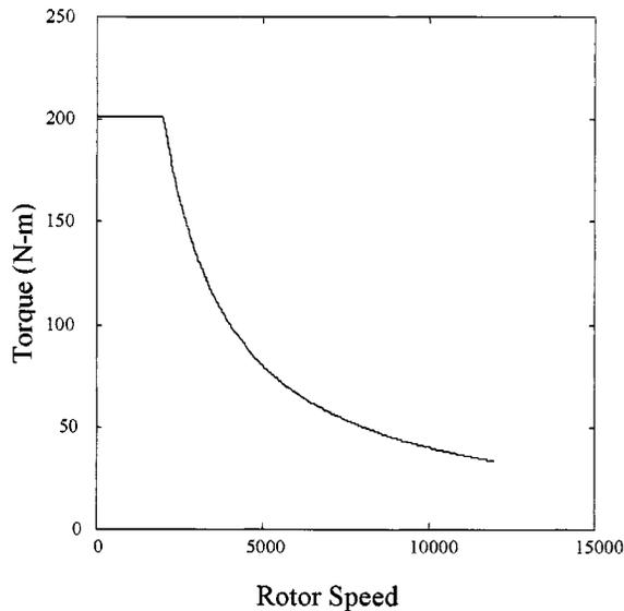
Fig. 2. Extended constant power range of SRM.
