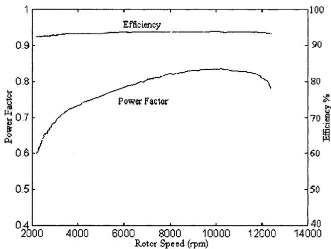
Fig. 3. Efficiency and PF of the SRM for constant power operation.
