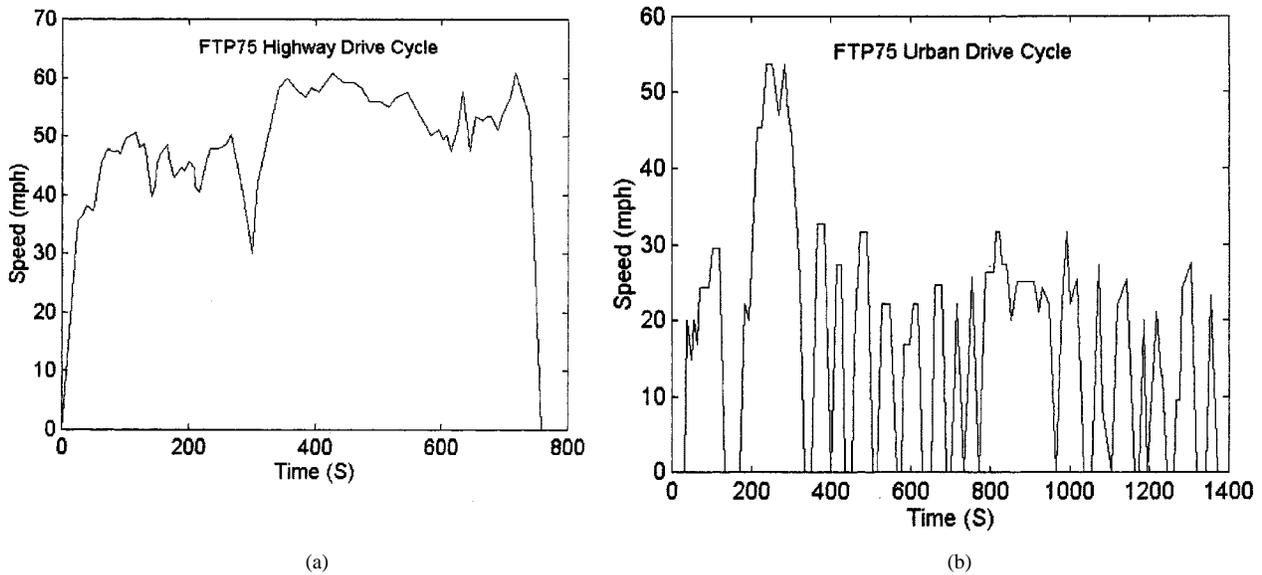
Fig. 5. FTP75 (a) highway and (b) urban drive cycles.
