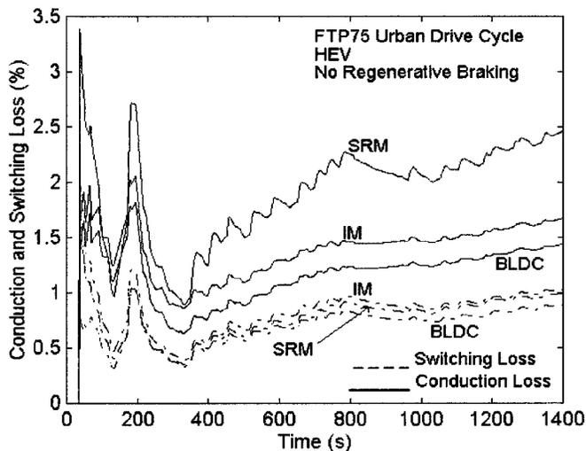
Fig. 7. Converter losses for HEV in urban drive cycle.
