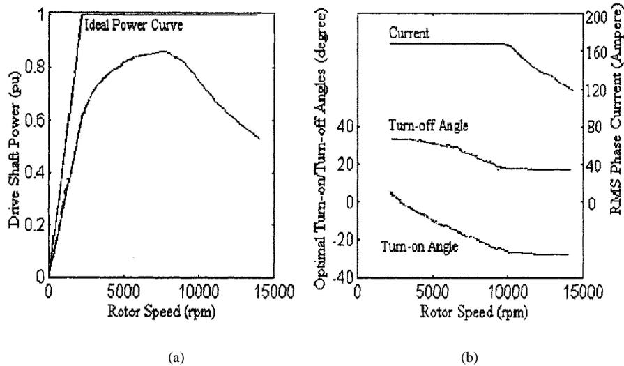
Fig. 4. (a) Maximum output power and (b) optimal control angles and rms phase current for the SRM design.
