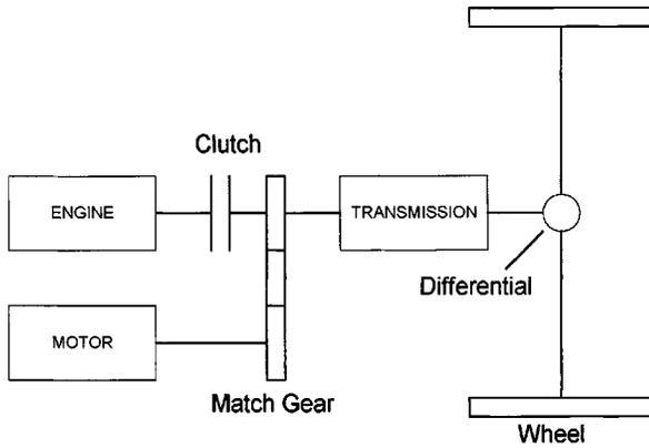
Fig. 1. Configuration of an electrically peaking hybrid (ELPH) vehicle [14].
