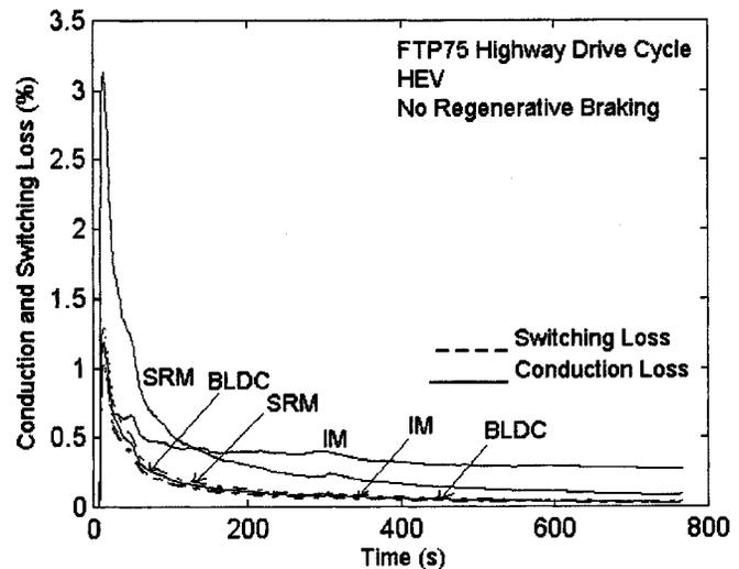
Fig. 8. Converter losses for HEV in highway drive cycle.
