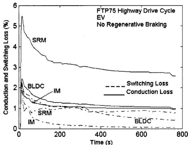
Fig. 10. Converter losses for EV in highway drive cycle.
